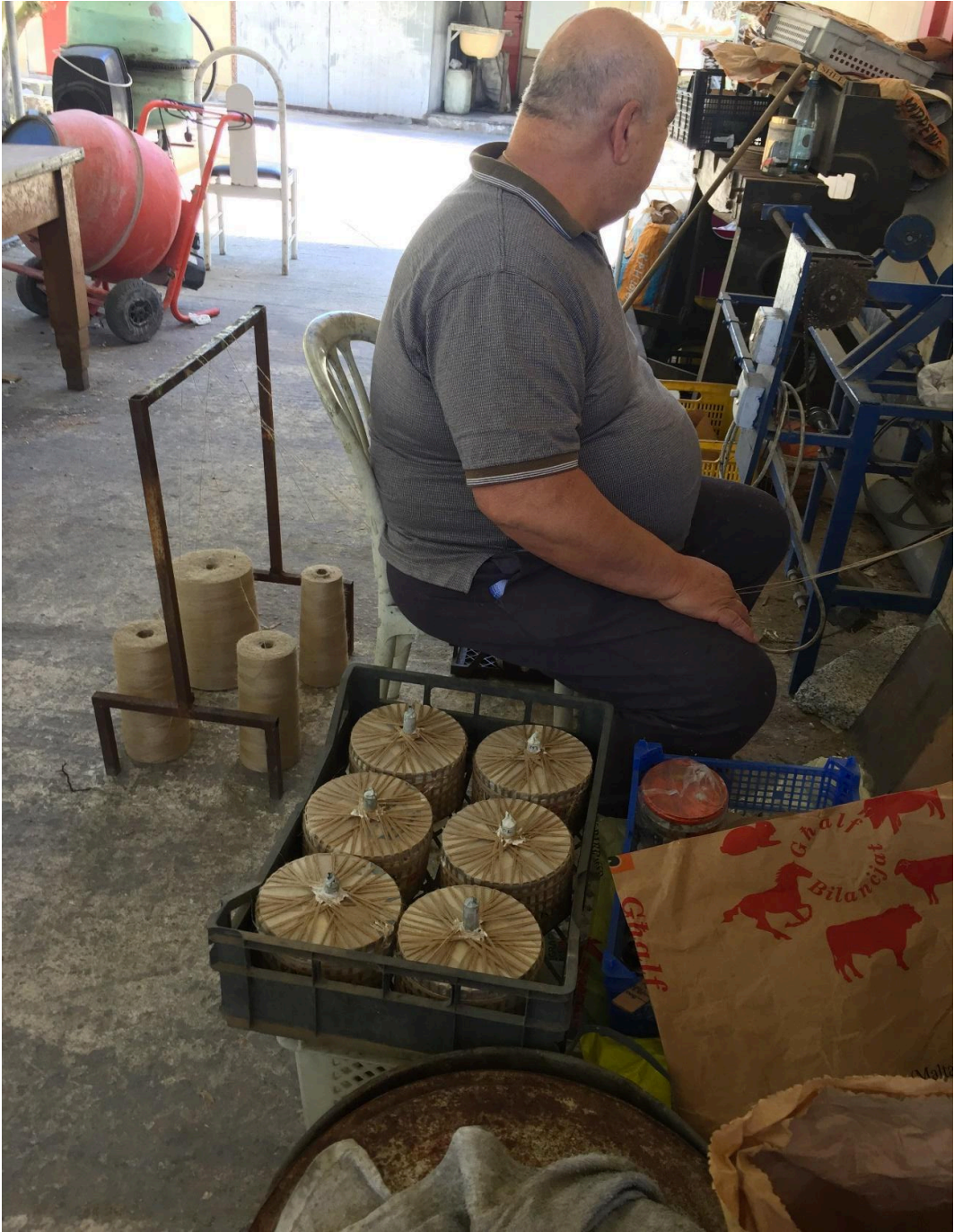
Shell spiking at the Gudja fireworks factory, Malta April 2023. Lotsa string. +10 points for using his butt to tension the string.
